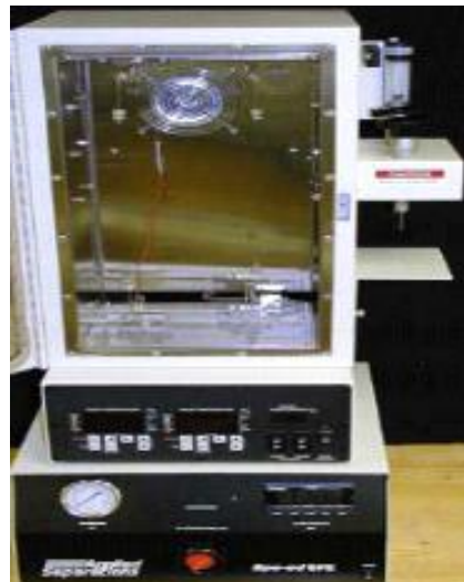
Bench scale SFE-CO 2 plant high view
